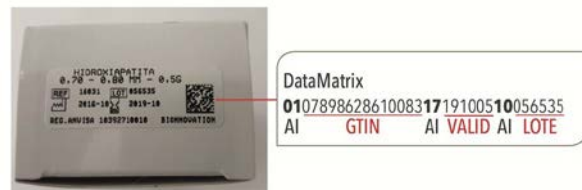
By using the GTIN in the GS1 DataMatrix the company complies perfectly with the FDA’s mandate.
