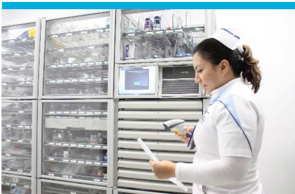
By scanning the GS1 DataMatrix barcode, a medication can be dispensed and tracked throughout the hospital to the point of administration to the patient.
