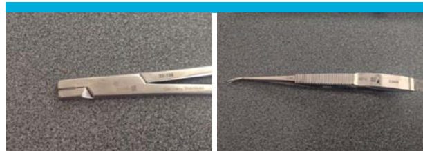
Each medical instrument is identified with a GS1 DataMatrix barcode for traceability through the sterilisation process.
