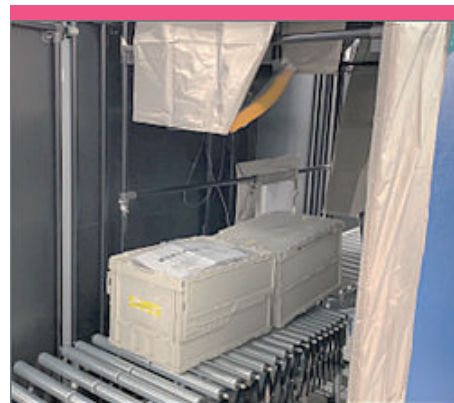
Figure 1.3.2.3.4-1 RFID Gate Reader
