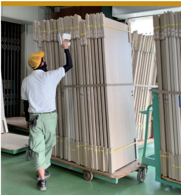
Figure 1.3.1.2-2 Reading RFID tags when shipping products from the factory
