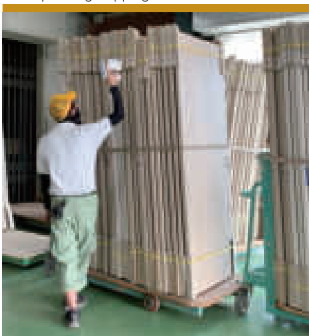
Figure 1.3.1.2-2 Reading RFID tags when shipping products from the factory
