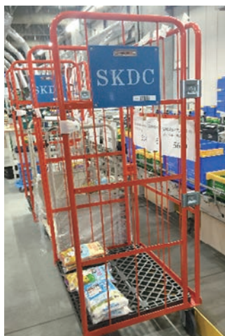
Fig. 1.3.1-3 Cage Trolley with an EPC/RFID tag on the destination board
