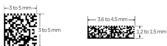
Fig. 1.2.2-2 Square and rectangular symbols of GS1 DataMatrix
