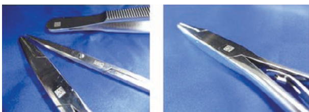
Fig. 1.2.2-1 GS1 DataMatrix directly marked on steel instruments
