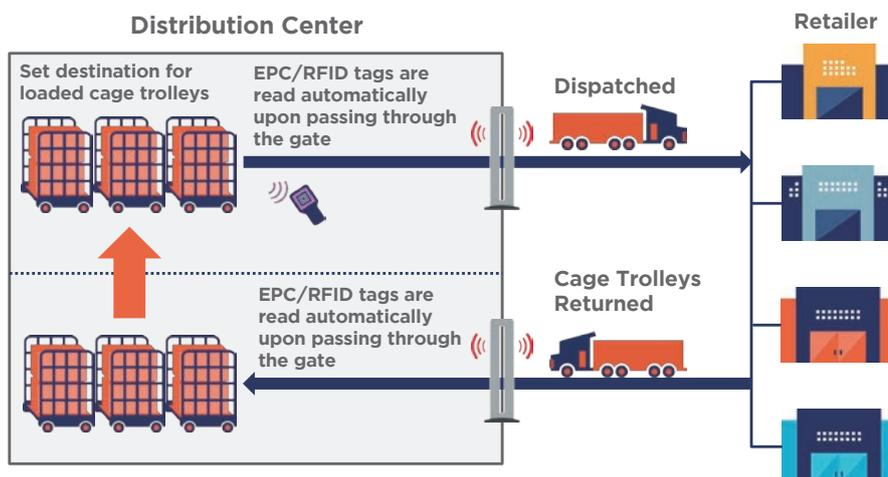
Fig. 3 Cage trolleys passing through the gate
