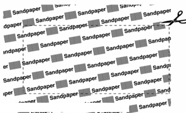
Figure 6.3.3.7-2. Barcode placement on random-wrapped item
