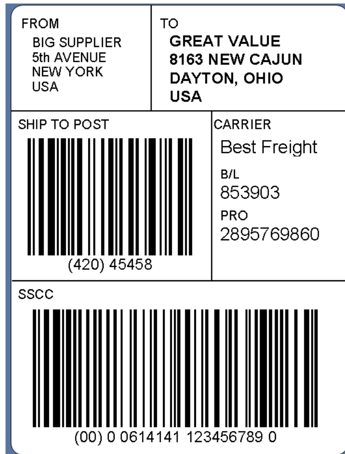
Figure 6.6.5-3. Label with supplier and carrier segments
