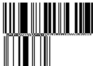
Figure 5.5.2.3.2-1. GS1 DataBar Expanded Stacked barcode
