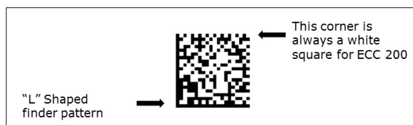
Figure 5.6.2-1. GS1 DataMatrix symbol
