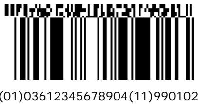
Figure 5.11.8-5. GS1 DataBar Omnidirectional symbol with a four-column CC-A
