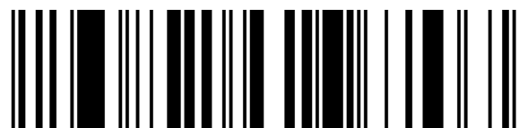
Figure 5.5.2.3.1-1. GS1 DataBar Expanded barcode
