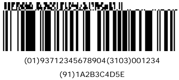
Figure 5.11.8-8. GS1 DataBar Expanded symbol with a four-column CC-A
