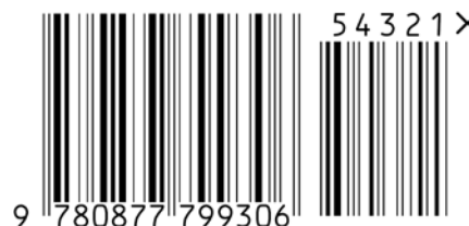
Figure 5.2.2.5.2-2. EAN-13 barcode with five-digit add-on symbol
