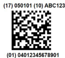
Figure 5.1-6. GS1 DataMatrix barcode
