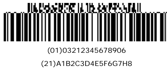
Figure 5.11.8-9. GS1-128 symbol with a four-column CC-A
