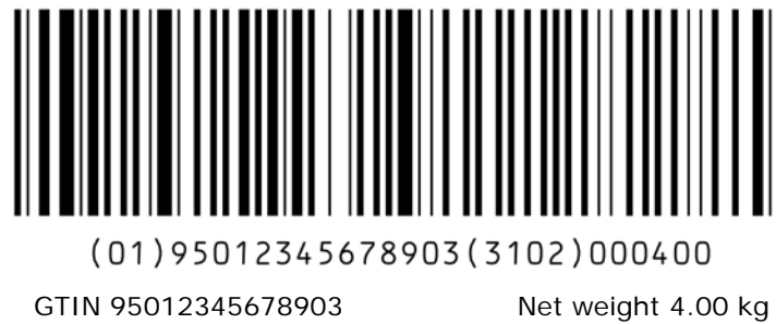
Figure 7.8.5.1-2. Data encoded in one concatenated GS1-128 symbol
