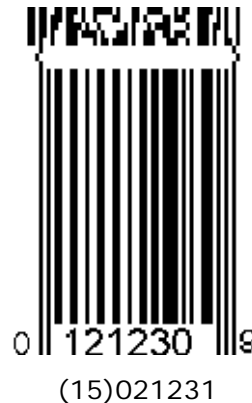
Figure 7.8.5.3-2. Example of mixed GS1 symbologies (GTIN encoded in UPC-E, Best before date in Composite)
