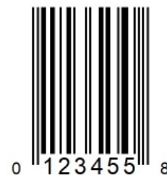
Figure 5.2.2.4-1. UPC-E barcode (encoding 001234000057 by zero-suppression)
