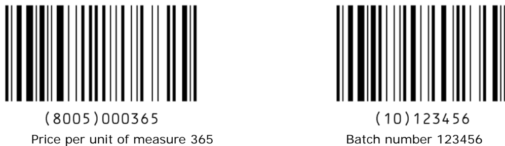
Figure 7.8.5.2-1. Data encoded in two GS1-128 symbols
