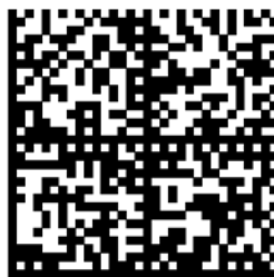
Figure 5.6.3.2-3. Segmented GS1 DataMatrix symbols: Square and rectangular formats (sizes of these GS1 DataMatrix symbols are larger than what would be used in a typical application so that typical alignment patterns can be easily seen.)
