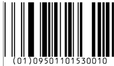
Figure 5.1-4. GS1 DataBar Omnidirectional barcode
