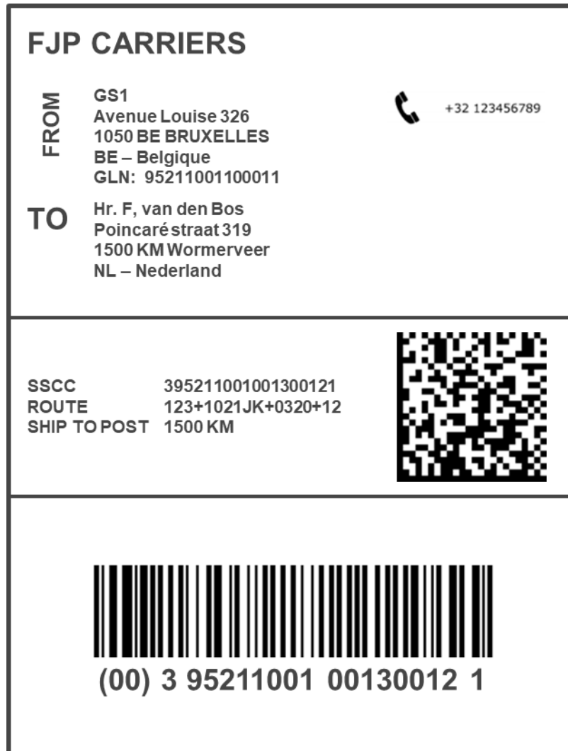
Figure 6.6.5-8 Label GS1 DataMatrix encoding transport process information
