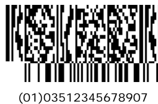
Figure 5.11.8-7. GS1 DataBar Limited symbol with a three-column CC-B
