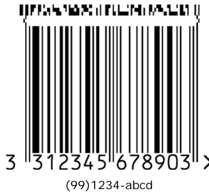
Figure 5.11.8-1. EAN-13 symbol with a four-column CC-A component
