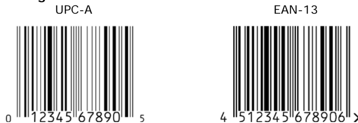
Figure 5.1-1. UPC-A and EAN-13 barcodes
