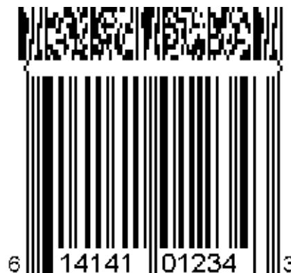
Figure 5.11.8-2. UPC-A symbol with a four-column CC-B component
