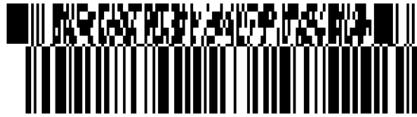
Figure 5.11.2-2. GS1-128 Composite symbol with CC-C
