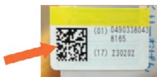
Figure 1.1.1.3-2 GS1 Data Matrix with the GTIN and the expiration dates
