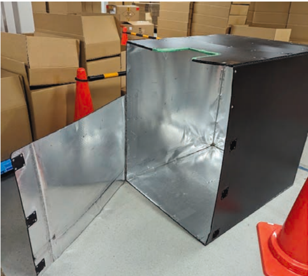
Figure 1.3.2.3-7 RFID Shielding Container for Inspections
