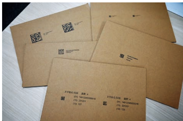
Figure 2.1.4-1 GS1 Data Matrix directly printed on cardboard cases
