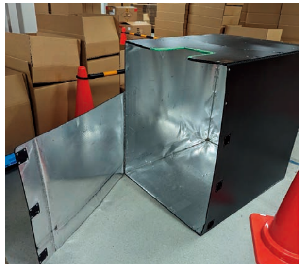
Figure 1.3.2.3-7 RFID Shielding Container for Inspections
