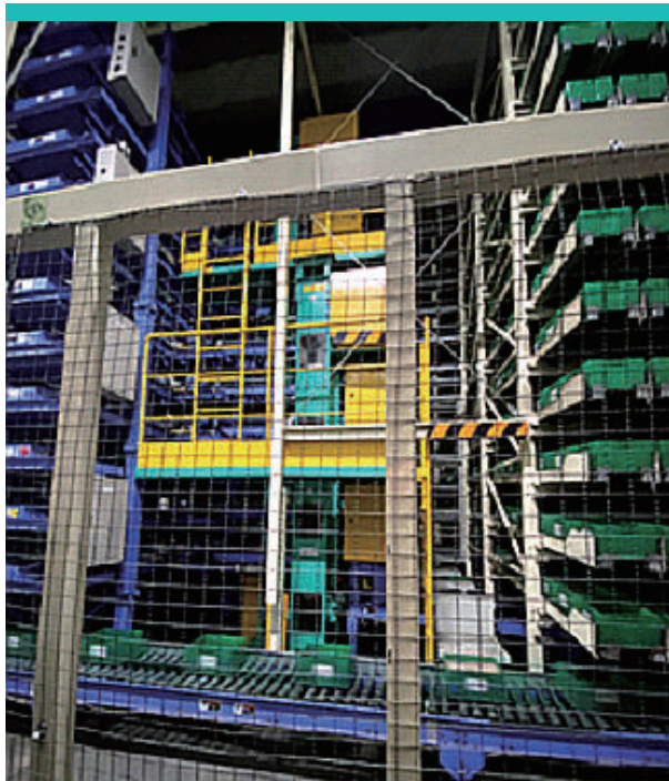
Figure 1.1.1.3-1 Automated storage rack
