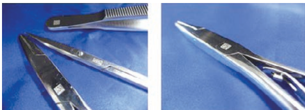
Fig. 1.2.2-1 GS1 DataMatrix directly marked on steel instruments
