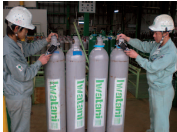
Fig 3.3.2-1 EPC/RFID operations at a gas cylinder filling station
