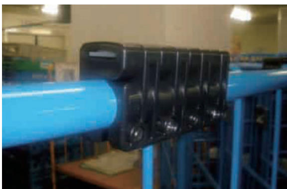
Fitting attachment for EPC tags
