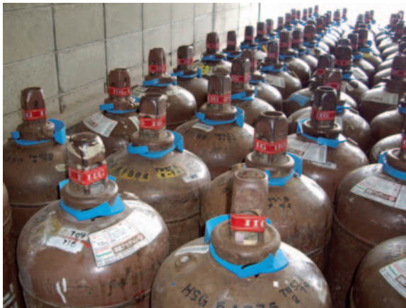
Fig 3.3.2-1 EPC/RFID operations at a gas cylinder filling station
