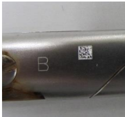
Fig. 4-11 Example of marking after 24-hour salt spray test
