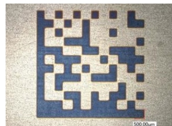
Cold marking technique
