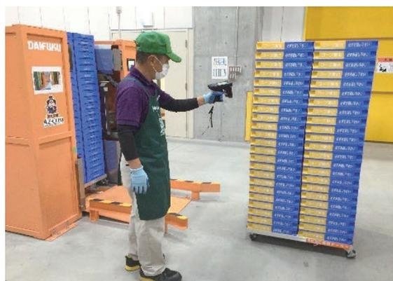
Returned foldable containers are scanned using a hand scanner.
